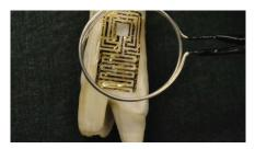
example, a graphene-based sensor printed on biodegradable silk is designed to be placed on a tooth to alert the wearer of dangerous bacteria in their saliva. In one test, it successfully identified a single E. coli microbe, and was able to pick out H. pylori (the culprit responsible for stomach ulcers) in human saliva.
