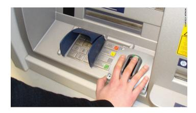
When exposed to near-infrared light, the hemoglobin in the blood appears as a pattern of dark lines. This pattern is recorded by a camera and compared to a database of registered images. Because the veins are located beneath the skin surface and the method only works on living persons, finger vein identification is almost impossible to counterfeit.
