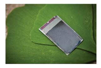
releases oxygen, and to a nickel-molybdenumzinc alloy on the other side, which releases hydrogen. When placed into a container of water and exposed to sunlight, the device generates two streams of bubbles that can be collected and stored as fuel to generate power. And unlike existing electrolysis systems, the device will even work in dirty water.
