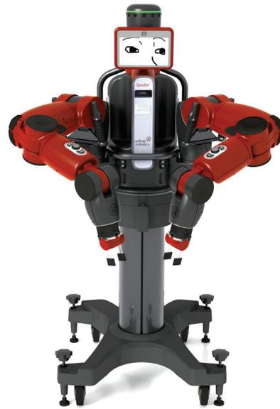
simply by moving one of his massive arms through the motions. Built-in sonar sensors and motors detect and respond to touch, making the limb light as a feather and just as easy to move. He can also be taught to recognize an object simply by holding it in front of one of its several cameras.
