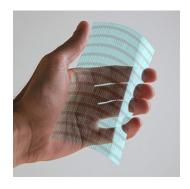
Graphene - sheets of carbon just one atom thick - has some pretty amazing properties. One hundred and fifty times stronger than steel and two hundred and fifty times more conductive than silicon, it's also pliable enough to be stretched to 120 percent of its length. But this latest research demonstrated something that hadn't been tested before - namely, graphene's ability to absorb an impact.
