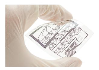
for manufacturers. Recently, however, researchers demonstrated a mechanically flexible sensor network that can be wrapped around irregular surfaces and visually map variations in pressure.
