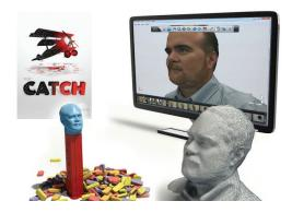
A free iPad app was recently released that's designed to make 3D printing easier than ever. Dubbed 123D Catch, it eliminates the need for costly and complicated rendering software. Users simply take pictures of the object to be rendered from different angles using their iPad. The images are uploaded to the Autodesk cloud service where they can be transformed into a 3D model. An identical copy of the original object can then be manufactured using 3D printing technology.
